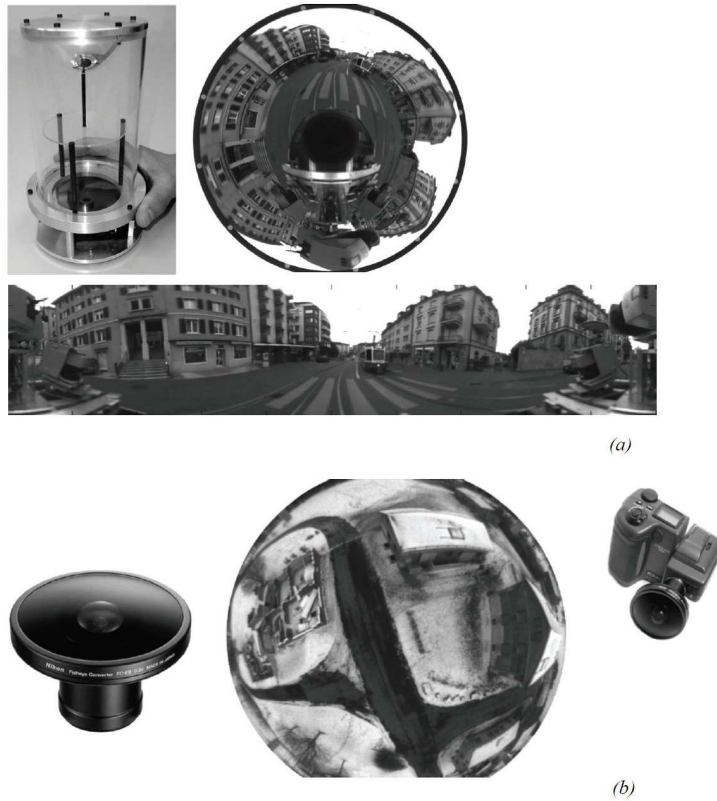
Figure 11: (a) A catadioptric omnidirectional camera using a hyperbolic mirror. The image is typically unwrapped into a cylindrical panorama. The field of view is typically 100 degrees in elevation and 360 degrees in azimuth. (b) Nikon fisheye lens FC-E8. This lens provides a hemispherical (180 degrees) field of view. [48]
